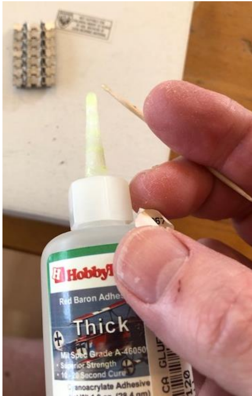
Figure 8: Apply a Small Drop of Glue to the End of a Toothpick
